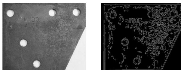
Fig. 8. (a) Image captured by the system (b) After the canny edge detection
